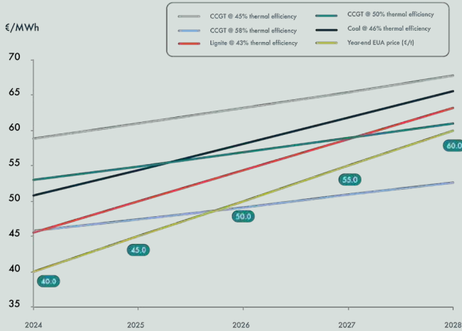
Figure 8: Stylized German merit order for fossil-fuel (FF) generators in a Paris-compliant scenario over 2024-28 with a range of CCGT efficiency rates, and with EUAs rising to €60/t by year-end 2028
