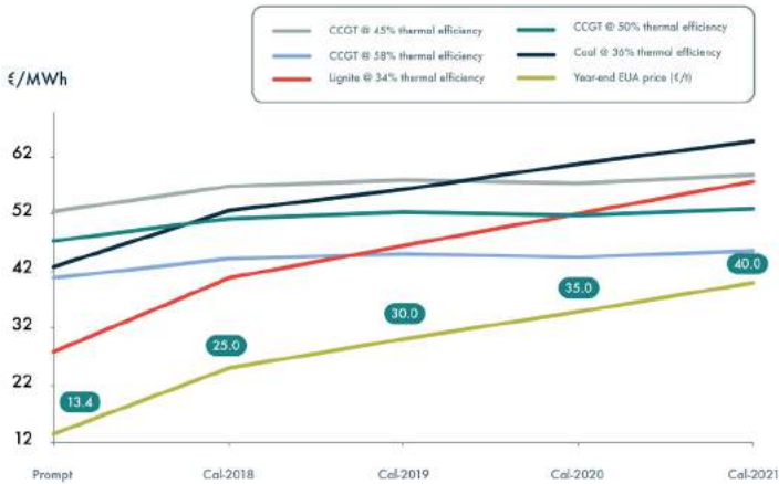
Figure 25: Stylized German merit order for FF generators with a range of CCGT efficiency rates, and with EUAs rising to €40/t by y/e 2021
